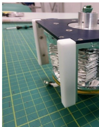
Packaged Inflatable; Combined Inflatable and Deployable Boom Mechanism
